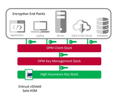
Entrust nShield HSMs safeguard and manages the cryptographic keys used by Randtronics DPM, providing a root of trust for the enterprise data privacy management program.
